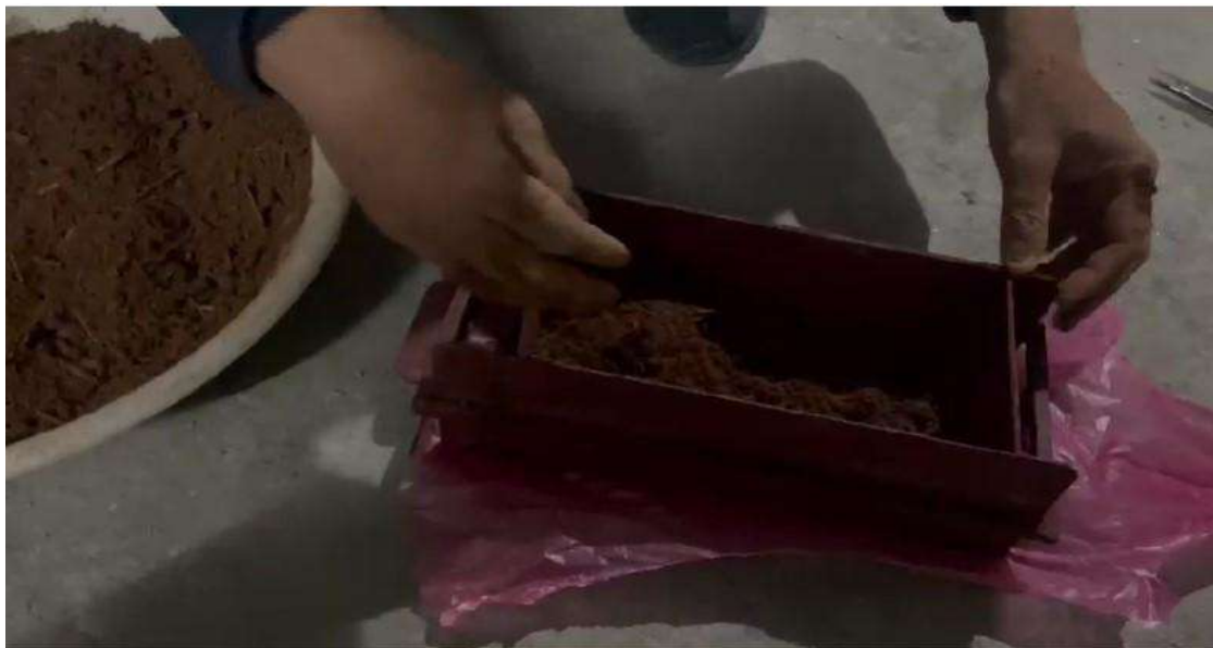
Figure 4: Placement of mixture in mould
