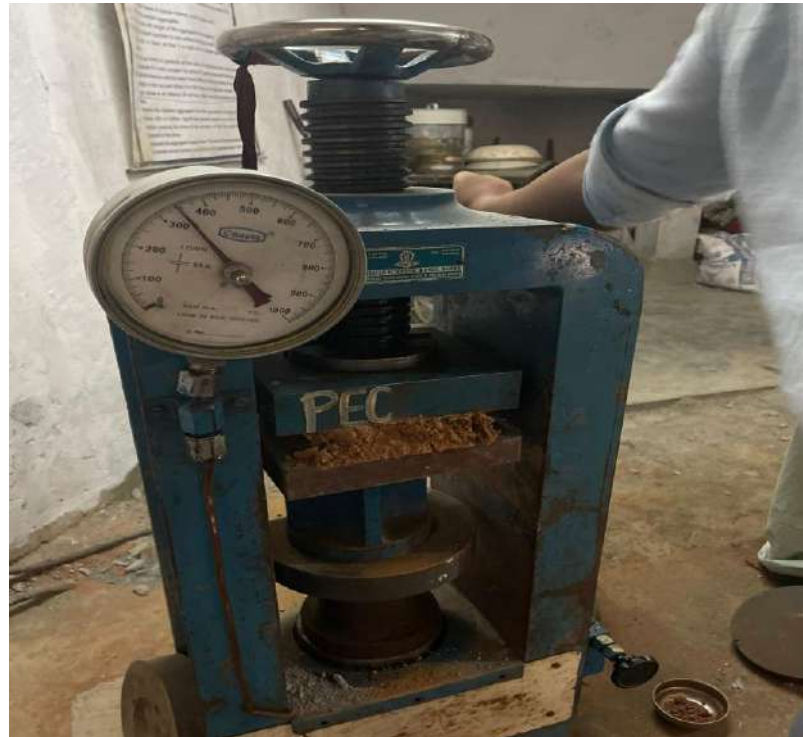
Figure 12: Compressive strength Test
